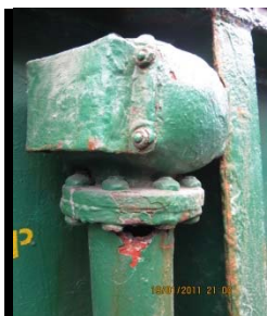
Picture 1 – Ballast Air Pipe Holed
