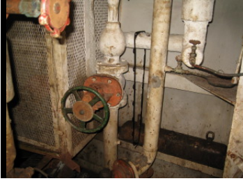
Picture 1 - Bilge discharge directly to the sea
