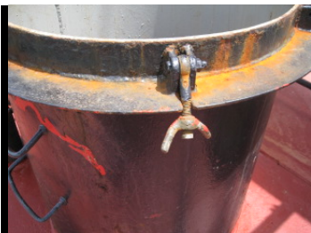
Picture 3 - Cargo Tank lid securing devices broken
