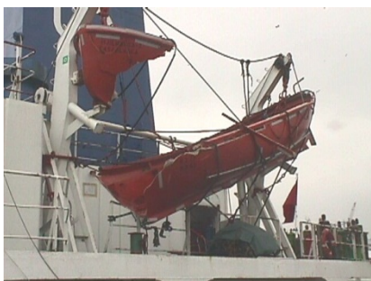
Picture 6 – Boat suspended in Davit
