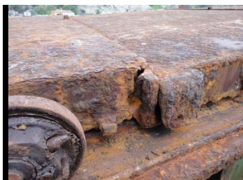
Picture 2 – Broken Damper
