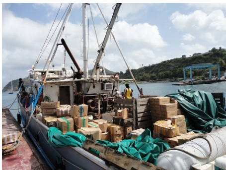
Picture 8 - Improper stowage of cargo and supplies
